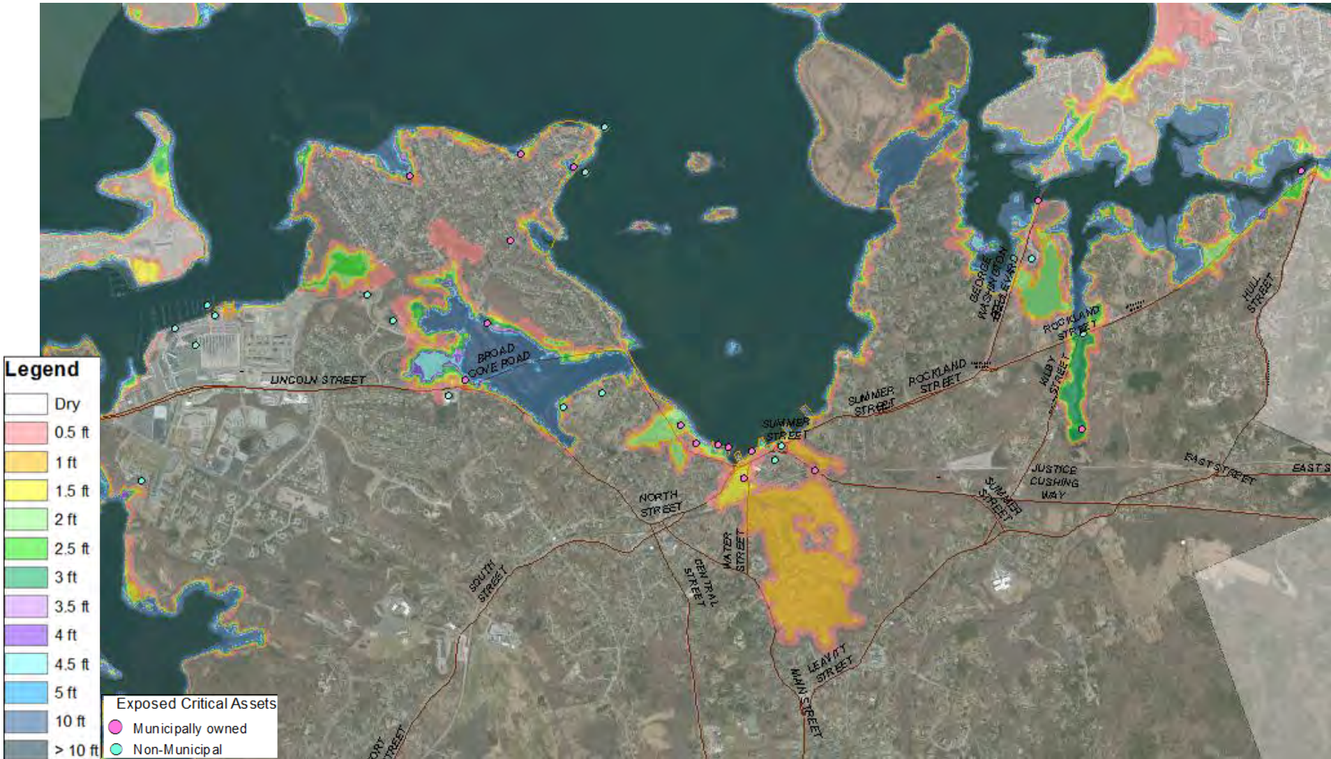
Depth of Flooding above Ground
